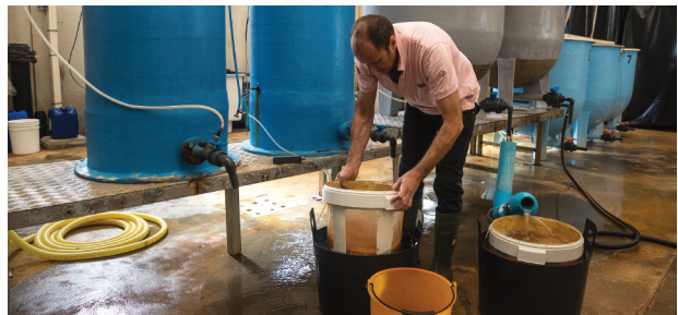
INVE Aquaculture's SEP-Art technology at work: the nauplii are separated from the shell by a set of passive magnets. What comes out of the separator pipe are pure, clean and active nauplii.
